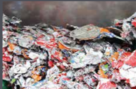
AL cans after dewatering
