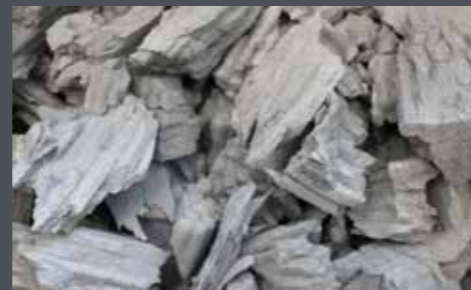
XPP insulation boards, crushed
